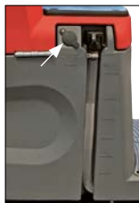
Fresh water drain hose with level indicator and opening for fresh water filler hose
