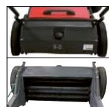
Adjusting screw for main brush
