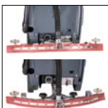
Suction nozzle lift- off with foot control
